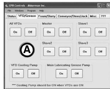
Cutterhead VFD Controls On Control Screen
