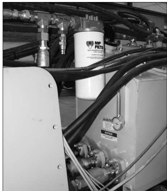
Rear Hydraulic Car #7 Hydraulic Fill & Main Reservoir
